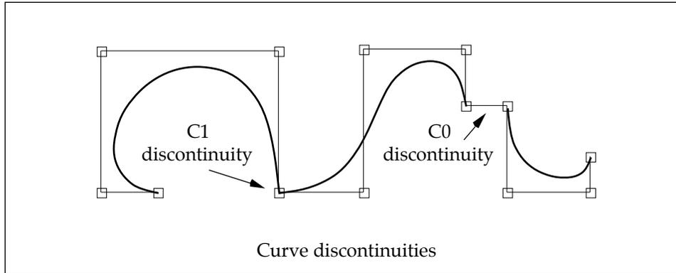
You get a  $C_n$  discontinuity in a curve if the knot vector contains the same value  $k-n$  times in a row.<sup>5</sup> For example, in the cubic curve above the knot vector is [0 0 0 0 1 2 2 2 3 4 4 4 4 5 5 5 5]. The  $C_1$  discontinuity occurs at 2 ( $k - 1 = 3$  two's in a row) and the  $C_0$  discontinuity occurs at 4 ( $k - 0 = 4$  four's in a row). You can use the knot insertion techniques discussed below to add discontinuities to curves.
