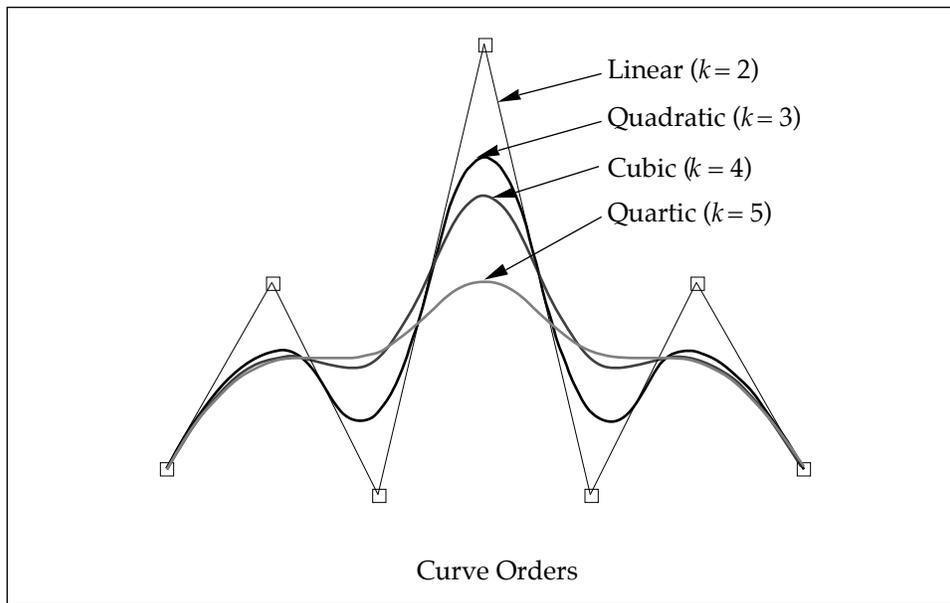
The effect of moving a particular control point depends on the order of the curve. If the order is high, moving a single control point affects more of the curve than if the order is low.
