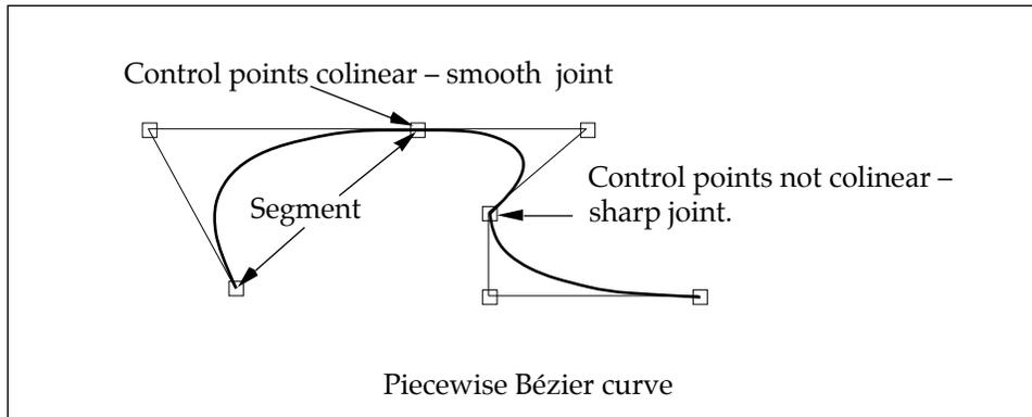
A quadratic piecewise Bézier knot vector with seven control points will look like this [0 0 0 1 1 2 2 3 3 3]. In general, in a piecewise Bézier knot vector the first  $k$  knots are the same, then each subsequent group of  $k-1$  knots is the same, until you get to the end. Note that a piecewise Bézier curve must have  $nk-1$  control points, where  $n$  is the number of segments (i.e., the number of control points is one less than an even multiple of the order).
