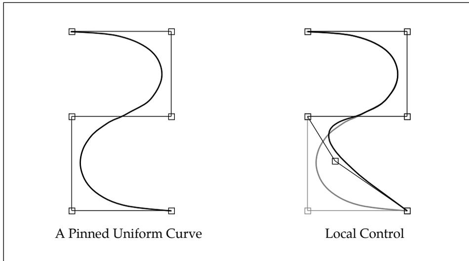
Just so you know what it looks like, here's the format of the pinned uniform knot vector. If  $k$  is the order, then the first  $k$  knots have the same value. Then the knots increase in uniform steps (usually by one) until we get to the last  $k$  knots which are also the same. So for the cubic ( $k = 4$ ) curve above, with six control points, the knot vector would look like: [0 0 0 1 2 3 3 3 3].
