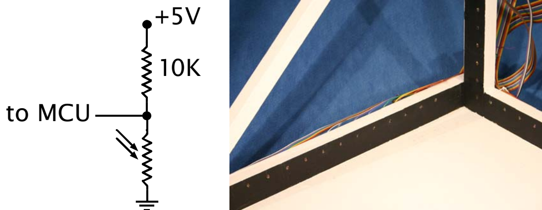
Figure 4 - Photosensor schematic, photosensors on the measurement frame
